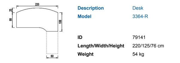
for extension on the right, Combi-worktop with laminate coating, worktop thickness 2.4 cm, plate on the operator side with rounding, radius 50 cm, visitor side in the middle 25 cm deepened and rounded, depth in the extension-area on the right 60 cm, 5-base apron framework of powder coated steel tube, base cross section round  $\emptyset$  50 mm, height-adjustable felt floor gliders  $\emptyset$  40 mm.
