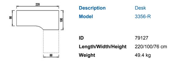
for extension on the right, Combi-worktop with laminate coating, worktop thickness 2.4 cm, plate on the operator side with rounding, radius 50 cm, depth in the extension-area on the right 80 cm, 5base apron framework of powder coated steel tube, base cross section round Ø 50 mm, heightadjustable felt floor gliders Ø 40 mm.
