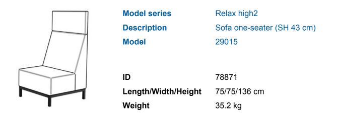
total height with high backrest and headboard 136 cm, seating surface height 43 cm. 4-base apron framework of square steel tube 30/30 mm, powder coated in RAL 9006 white aluminum, linking devices, felt floor gliders.
