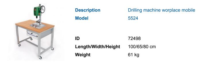
Machine bench: Dimensions 100/65/80 cm, worktop and lower shelf of glued plywood (beech), frame of square steel tube, feet of shaped tube 60/60/2 mm, frame of shaped tube 40/40/2 mm, powder coated, 4 swivel castors Ø 75 mm, lockable castors, lockable sheet drawer.
