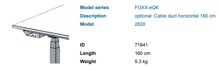
additional equipment for electrically height-adjustable desks with worktop length 160 cm, cable duct 142/19 cm made of sheet steel, with side suspensions, fold-down on both sides, powder coated in silver.
