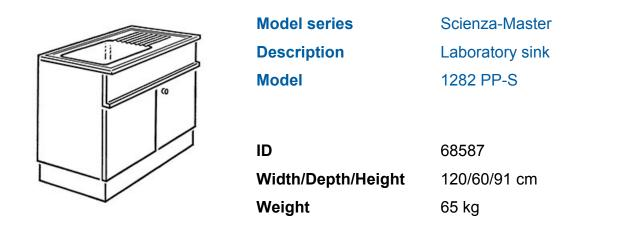
120/56(60)/91 cm Sink with drainboard of polypropylene 120/60/4 cm, basin made of polypropylene on the left or right, interior dimensions 40/40/25 cm, at the top a sink cover 20 cm high, underneath 2 revolving doors with drilled stop damping, aperture angle 270°, hinges powder coated with automatic hold-closed function, cylinder locking device with olive handle, waste collector, fitted shelf, plastic plinth panel with bottom-sided sealing lip.
