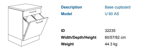
with waste organiser, on top 1 drawer, below front plate for full extension with kick automatic. **Equipment:** 1 waste-sorter, approx. 56/50/40 cm, Franke, Typ 700 K 60 KickMatic, item no. 907 220 000, with manual extension and foot kick system, full extension incl. 2 waste bins each 18 litres capacity and 2 waste bins capacity 8 litres each, all containers with carrying handle.
