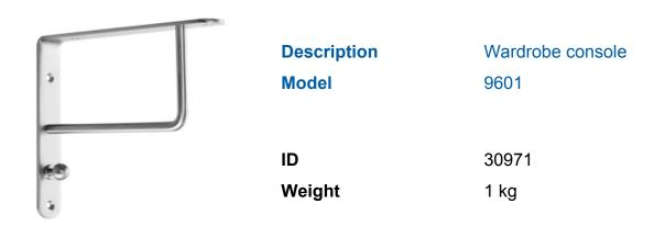
30/250/200 mm, of steel, surface stainless steel effect, outreach 250 mm, with coat hooks and connecting bracket for coat hangers, screwed to the back panel / wall covering.
