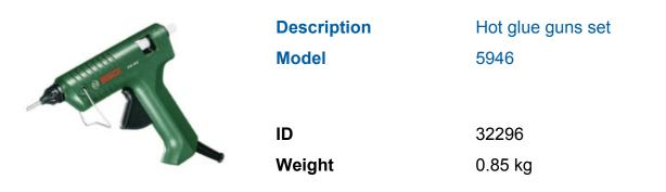
electronically controlled heating elements for fast commitment and constant working temperature, hot-melt adhesive preheating, mechanical feed for sensitive dosing, hot-melt adhesive guide with viewing window, anti-drip device, long nozzle, support mechanism for a secure stand, on/off indicator light, adhesive performance 20 g/min, hot-melt adhesive-Ø 11 mm, hot-melt adhesive-length 45 to 200 mm, incl. 500 g glue sticks.
