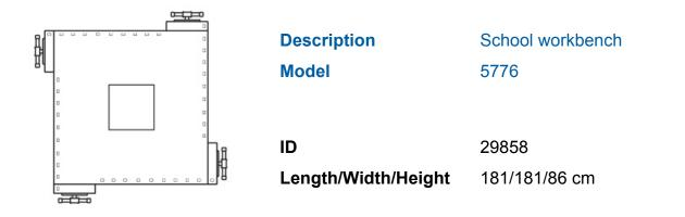
four-seated, 181/181/86 cm, heavy finishing, 4-base wooden framework, worktop 9 cm thick, completely manufactured of solid and chamber-dried beech wood, surface impregnated with linseed oil varnish, tool rest deepening (35/35 cm) in the worktop.
