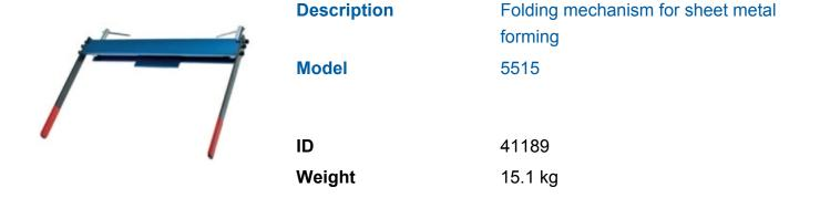
working width 630 mm, for machining of sheet components (sheet steel 1.2 mm, aluminium sheet 1.5 mm), repeated possibility fold with various distances, easy and rapid extraction of a closed profile by fast removing a toggle screw, prepared for clambing in the parallel-vice.
