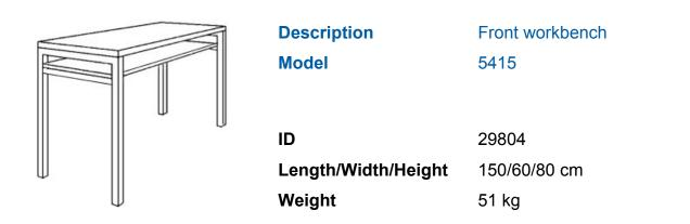
150/60/80(70) cm, worktop of glued laminated plywood (multiplex board), board thickness 3.5 cm, oiled, tray, 4-base apron framework of square steel tube 60/60/2 mm, relocated longitudinal aprons (mounting of vices), with height-adjustable felt floor gliders Ø 40 mm.
