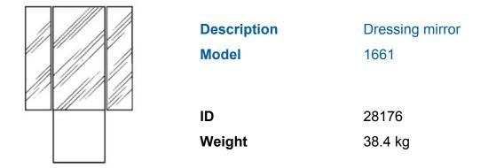
three-part, the middle mirror 60/120 cm, fixed to the wall, the both side mirrors, each 30/120 cm, as wings for opening and closing, carrying construction with support substructure.
