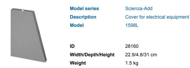
Cover for electrical equipment (left) 1598L, lockable, 23/4.8/31 cm, for the protection of the electrical equipment on the lectern shaped energy cell of the student's energy profile. Cover trapeze shaped, beveled on 3 sides (open at the bottom), of powder coated sheet steel, sheet thickness 1.5 mm, cover attachable to the mounting frame from above and lockable with cylinder lock. Incl. suspension device for electrical cover, fastened to the student's energy profile on the sides.
