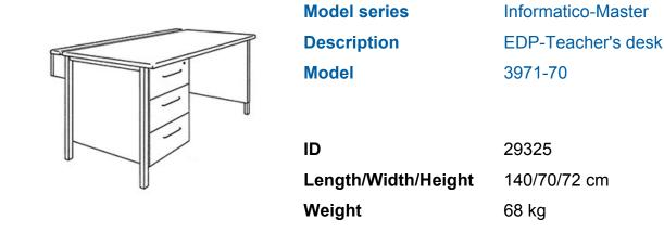
Desktop 2.4 cm thick, with 1 mm laminate coating, cable duct with folding cover on the long side, on the left base cupboard 45/52/57 cm, 3 synthetic drawers, top drawer with cylinder locking device, metal bow handles, privacy screen at the front and on the side, 4-base apron framework of powder coated square steel tube, base cross section 30/30/2 mm, adjustable synthetic floor gliders. Further dimensions and quality features accoring to ÖNORM A 1650.
