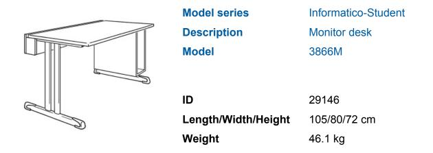
105/80/72 cm, with sliding desktop, desktop 2.5 cm thick, melamine resin coated on both sides, sliding desktop fixable, underneath cable duct across the whole table width, cable duct accessible through sliding of desktop, below desktop on the right or left a tower corpus with inner clearance 24/56/47 cm, double-base skid framework of powder coated oval steel tube, anti-slip protection floor gliders with taring gliding screw. Further dimensions and quality features according to ÖNORM A 1650.
