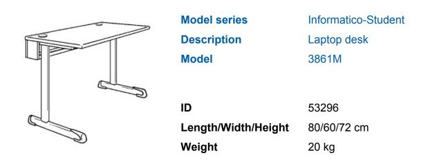
single-seated, 80/60/72 cm, desktop 2.5 cm thick, melamine resin coated on both sides, 1 cable jack with cover, underneath cable duct across the whole desk width. Skid framework of powder coated oval steel tube, anti-slip protection floor gliders with taring gliding screw. Further dimensions and quality features according to ÖNORM A 1650.
