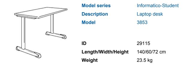
two-seated, 140/60/72 cm, desktop 2.4 cm thick, with 1 mm laminate coating, Skid framework of powder coated oval steel tube, anti-slip protection floor gliders with taring gliding screw. Further dimensions and quality features according to ÖNORM A 1650.
