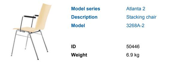
with armrests, 4-base round steel tube framework, Ø 18 x 2 mm, framework surface chromium, armrest soft grip hose black, stacking gooves, floor gliders with felt gliding surface. Beech plywood shell approx. 10 mm thick, glued 9-fold, shell in straight shape and with straight back top edge, back ergonomically shaped. Load test according to DIN 68878. **Stackability:** max. 20 chairs.
